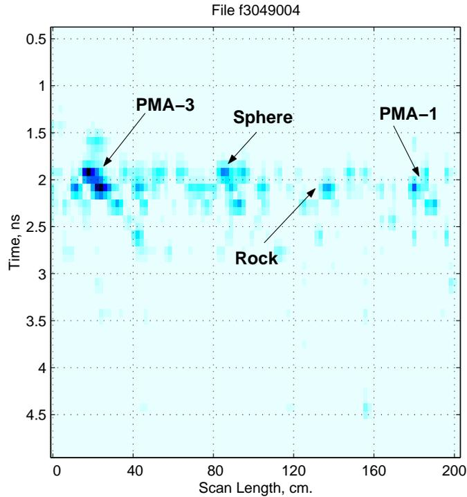
**Figure 8.** Best Basis Results With TUI Frequency-Stepped GPR
