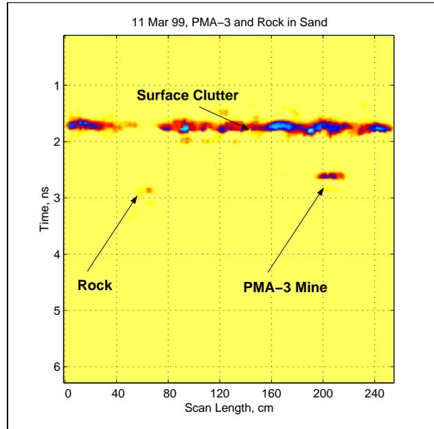
**Figure 5.** Wavelet Approach, Suppression of False Target
